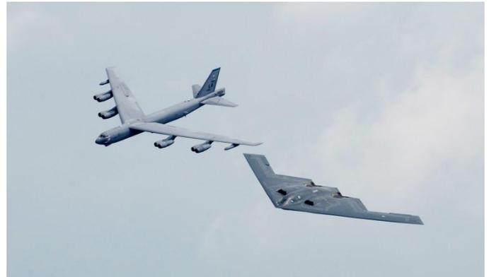
The largely composite B-2 has vastly reduced infrared, acoustic, electromagnetic, visual and radar signatures, extraordinary aerodynamic efficiency, a long range (6000 miles) without refueling and a massive payload. It is hence a potent delivery system for the likes of the MOP, as it is very difficult for defensive systems to detect, track and engage.
