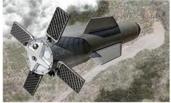
The MOP is deployed from high altitude and allows gravity to add momentum to its 30,000 pound weight so that it hits with sufficient kinetic energy to bury itself 200 feet underground and penetrate hardened concrete, then it explodes its 5,300 pound warhead.
