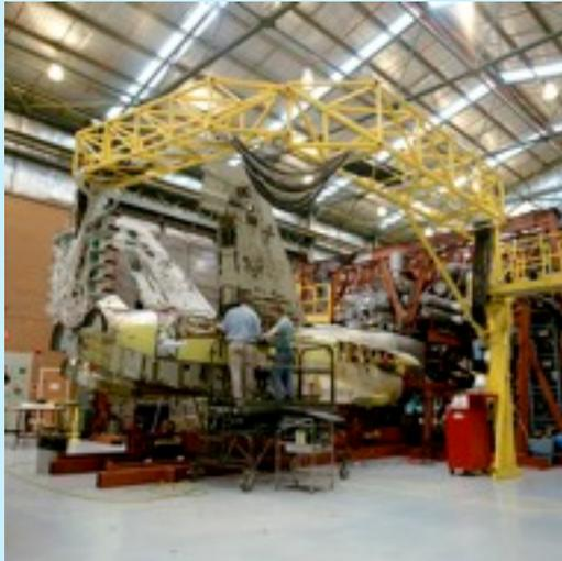
*Structural Fatigue Test of the F/A-18*
